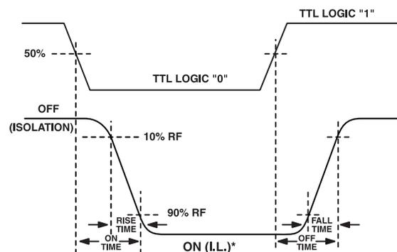
Figure 3 - Detected RF Power
