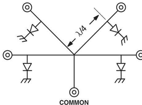
Figure 2b - Series Diodes at Common Junction
