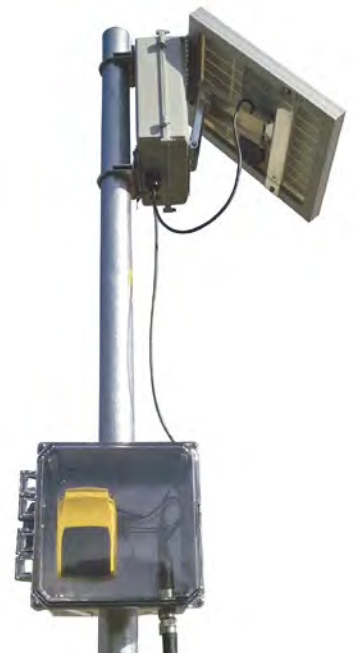
NBM-580 / NS3 System: NS3 in solar powered outdoor enclosure (right) remotely connected to NBM-580 (left)
