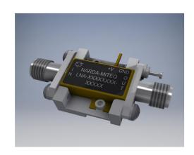
The ULNA amplifiers use InP-based HEMTs to enable the ultra-low noise performance and leverage Narda-MITEQ's extensive expertise with design and fabrication of low-noise amplifiers for highfrequency applications in challenging applications and harsh environments.
