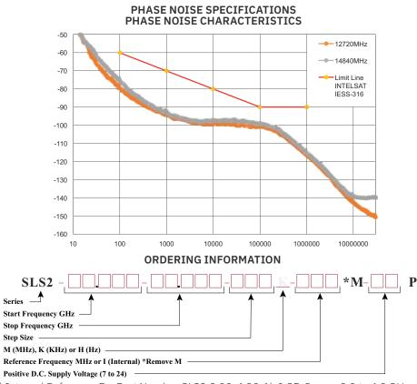
\* Internal Reference Ex: Part Number SLS2-2.00-4.00-1k-I-8P. Covers 2.0 to 4.0 GHz with a step size of 1kHz, has an internal reference and +8Volt supply.
