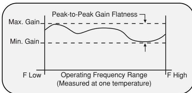
The gain flatness of a fiber link is measured by viewing the swept gain and determining the difference between the minimum gain and the maximum gain
