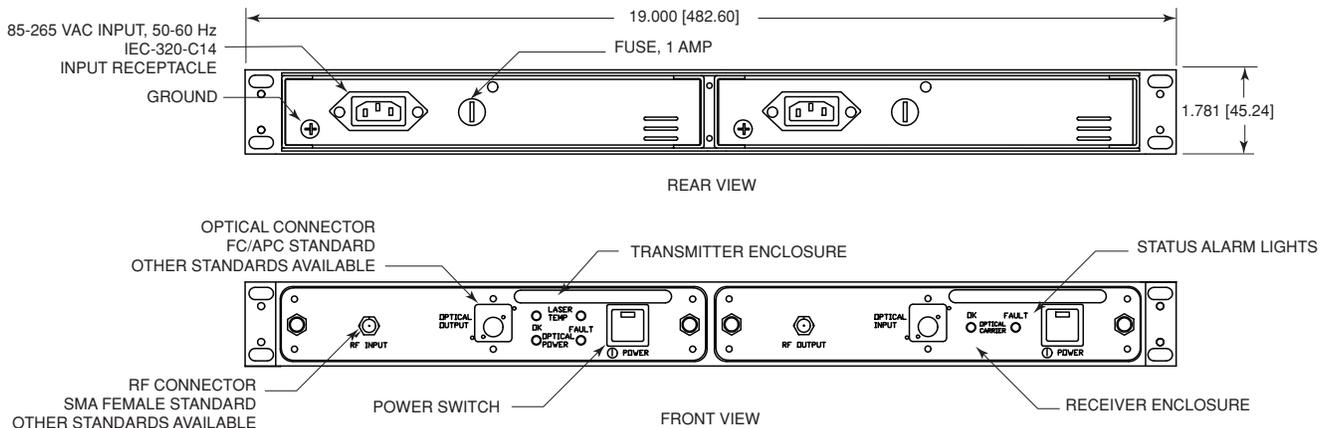
NOTE: PANEL MARKING AND STATUS LIGHT CONFIGURATION VARY WITH MODEL.
