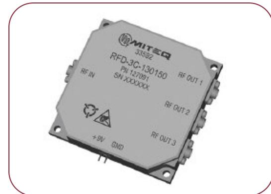
MITEQ's Model RFD-3C-130150 is an RF distribution module that receives an RF signal and distributes it to three different output ports. The signal goes through a two-stage amplifier and bandpass filter to provide an output that has low spurious and minimum harmonic content. This unit was designed for use in an extreme environment. It is small in size, lightweight, hermetic and has minimal DC power dissipation.
