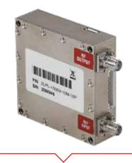
The L3Harris 2LPL Series phase-locked source offers excellent phase noise and spurious performance in a miniature 2.0" width x 2.0" length x 0.61" height housing and is available in fixed frequencies from 10 MHz to 15 GHz. Units can operate from either external reference, or internal TCXO with stability as low as 500 PPB. Flexible internal DC regulators allow operating DC from +7 VDC to +28 VDC.
