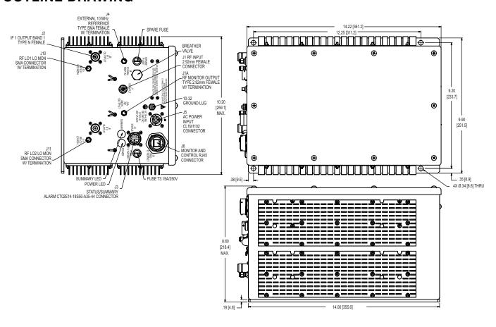
Note: Dimensions shown are in inches and those shown in brackets [ ] are in millimeters.
