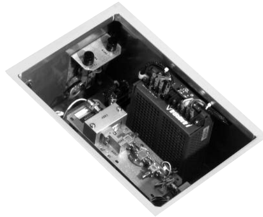
This small self-contained temperature stabilized Ka-band noise source was provided for offline system testing.
