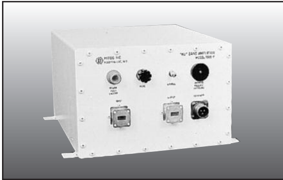
This small self-contained temperature stabilized Ka-band noise source was provided for offline system testing.
