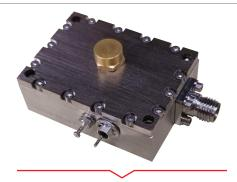
The Narda-MITEQ LCDRO is a free running DRO that is used in many microwave radar and radio frequency applications for both commercial and military.
