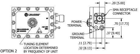
Note: Dimensions shown are in inches and those shown in brackets [] are in millimeters.
