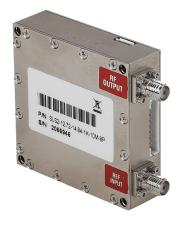
Narda-MITEQ SLS2 Series of high spectral purity synthesizers offer a low price alternative for L, S, C and Ku-bands with the lowest phase noise. With standard 1 kHz step size output at all bands the SLS2 series synthesizers are ideal for dual conversion up and down converters. With +13 dBm output power and 60 dBc spurious suppression, the SLS2 series support the most stringent system applications. Consuming less than 4 Watt maximum from (+7 to 28 V) DC supply.
