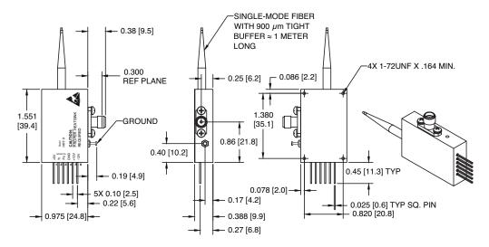
Notes: Dimensions shown are in inches and those shown in brackets [ ] are in millimeters. Unit weight is approximately 65 grams.
