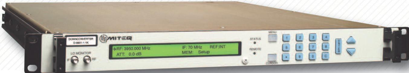
The MITEQ AFC frequency/block converters provide automatic frequency control to maintain communication links for Satellites with decaying or orbital perturbations. A 5 MHz AFC reference with a frequency deviation of  $\pm 60$  kHz is applied to the converters to compensate for frequency shift caused by Doppler effect. The resultant output frequency of the converter will be fixed to better maintain the communication link.
